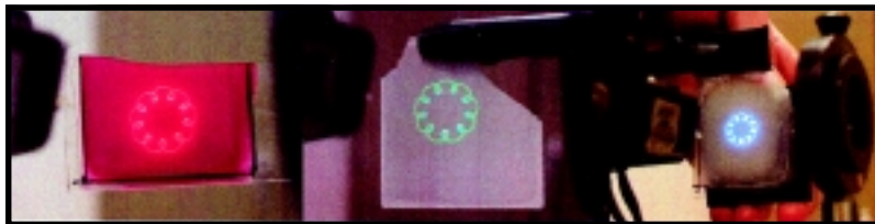
Figure 1 Examples of our red, green and blue emitters using up-conversion in rare earth doped fluoride crystals excited by diode laser light near 976 nm for the red and green and 959 nm for the blue. The red emitter is in a polymer containing a green absorbing dye that absorbs some unwanted green emission from this material.
