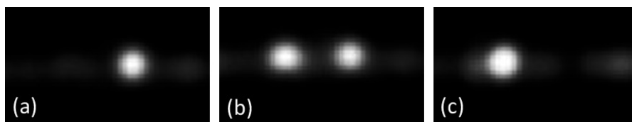
Figure 4.3. Optical power distribution of MZI's two output channel at a) I=0mA, b) I=0.67mA and c)1.47mA.
