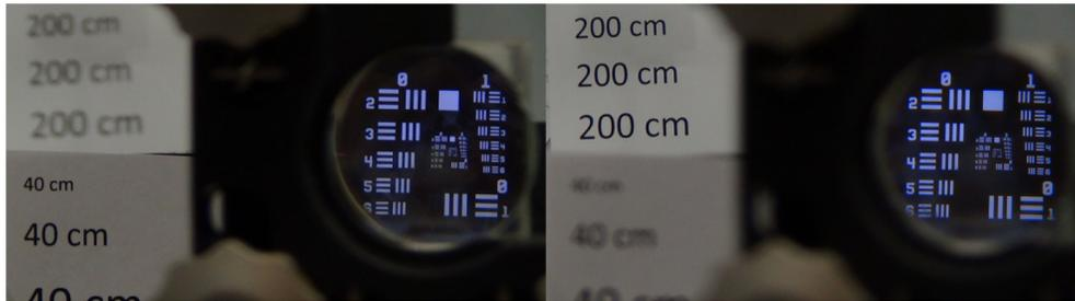
Fig. 4. When looking into the PBS, the switching between two paths results in different images as shown above. The left photo shows the image when the light travels through the shorter path, with the image being 40 cm away from the camera, while the right photo shows the image when the light travel the longer path, with the image being 200 cm away. Only one lens with  $f$  being 25 cm was used.
