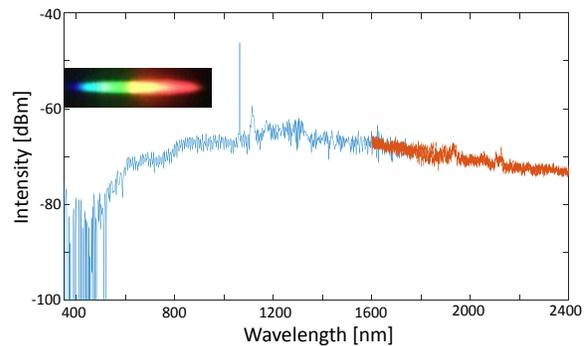
Fig. 2 Experimentally observed SC spectrum in a tapered parabolic multimode fiber with an NA=0.21. The data was collected using two different spectrometers. In all cases, the spectrum is homogenized as a result of tapering. The visible part of the spectrum is also depicted in the inset.
