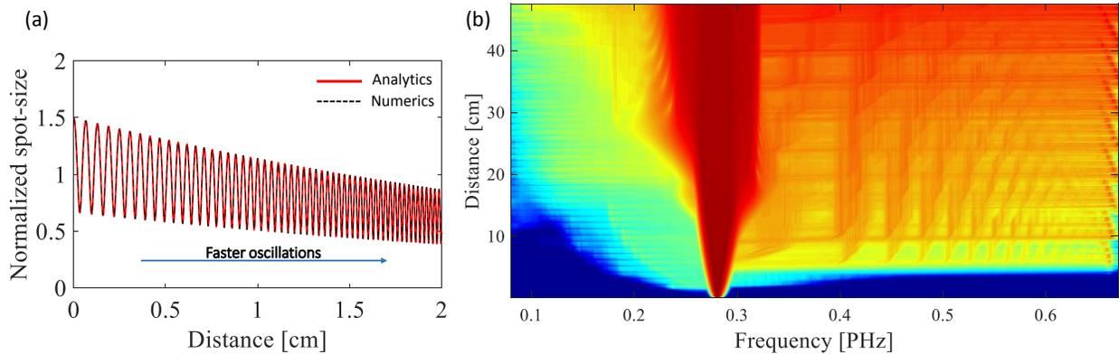
Fig.1 (a) Accelerated beating dynamics in a tapered multimode parabolic optical fiber. (b) simulated SC generation in a tapered parabolic fiber, when excited at 1064 nm. A continuous drift of the sidebands towards higher/lower frequencies is clearly observed.
