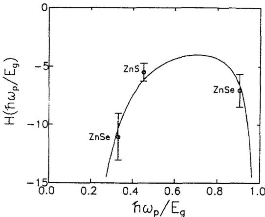
FIG. 13. A plot of  $H(x)$  versus  $x$  showing free-carrier refraction for three semiconductors as compared with theory (solid line). Figure from Wang *et al.* (1994).
