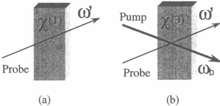
FIG. 2. (a) Linear system, material only, probed at  $\omega'$  to determine the linear absorption spectrum. (b) The system is now the material plus strong light beam at  $\omega_b$ , probed at  $\omega'$ , to determine the changed "linear" absorption spectrum.
