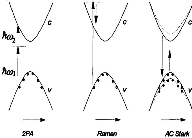
FIG. 3. Graphic representation of the processes involved in the nonlinear absorption in a two-band model. The small circles denote bound electrons.
