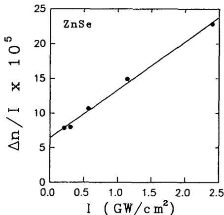
FIG. 12. A plot of the ratio of the change in refractive index to irradiance as a function of irradiance for 532-nm picosecond pulses in ZnSe. Figure from Said *et al.* (1992).
