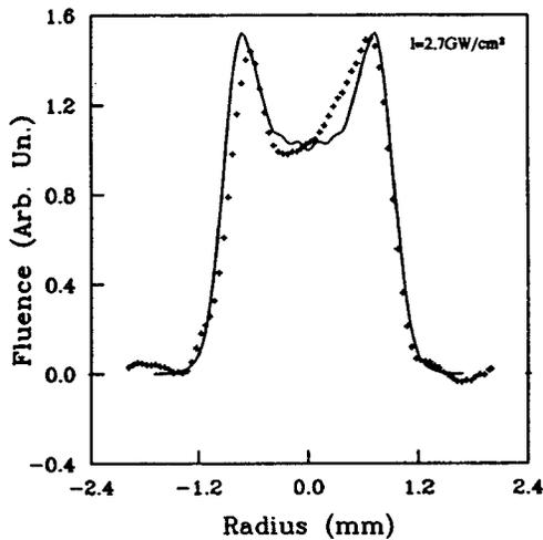
FIG. 15. A one-dimensional spatial profile in the near field of a picosecond 532-nm pulse transmitted through ZnSe. Figure from Van Stryland (1996).
