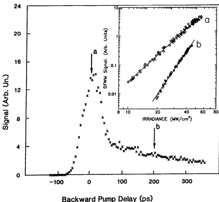
FIG. 17. DFWM signal in ZnSe for temporally coincident, copolarized, forward pump, and probe as a function of the time delay of the perpendicularly polarized backward pump. The inset shows a log-log plot of the output signal as a function of the input (all three inputs varied) for (a) zero temporal delay and (b)  $\sim 200$ -ps delay. Figure from Canto-Said *et al.* (1991).
