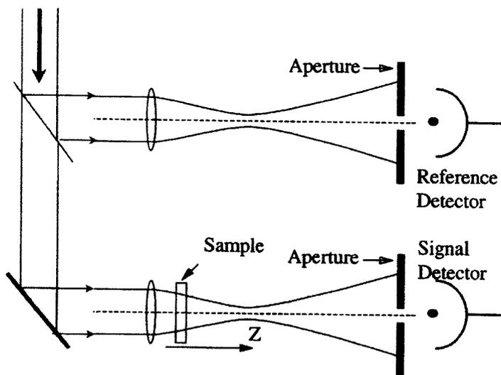
FIG. 18. Z-scan geometry with reference detector to minimize background and maximize the signal-to-noise ratio. Figure adapted from Sheik-Bahae *et al.* (1989).
