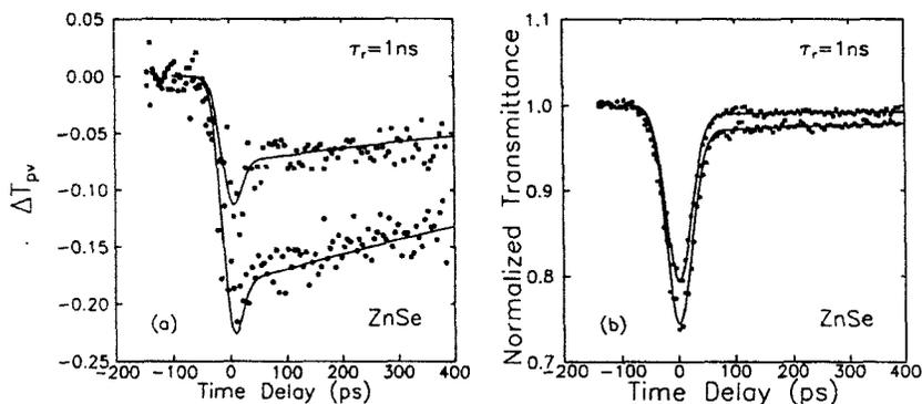
FIG. 23. Time-resolved Z-scan data on ZnSe using 532-nm, picosecond excitation pulses and probing at 1.06  $\mu\text{m}$ : (a) nonlinear refraction versus temporal delay; (b) nonlinear absorption versus temporal delay. Figure from Wang *et al.* (1994).
