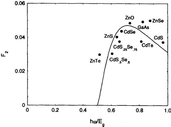
FIG. 5. The degenerate 2PA spectral function  $F_2(\hbar\omega/E_g)$  along with data scaled according to Eq. (51). (Data using transmittance from Van Stryland *et al.*, 1985b.)
