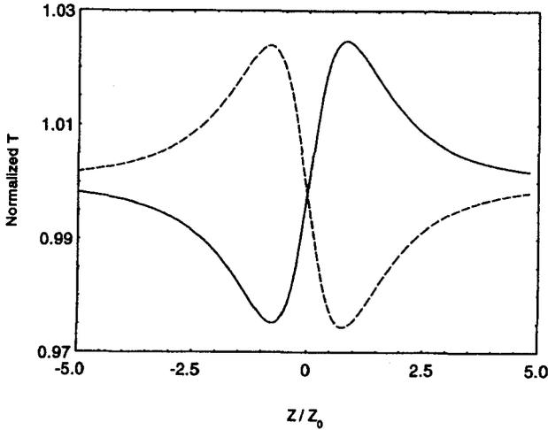
FIG. 19. Predicted Z-scan signal for positive (solid line) and negative (dashed line) nonlinear phase shifts.
