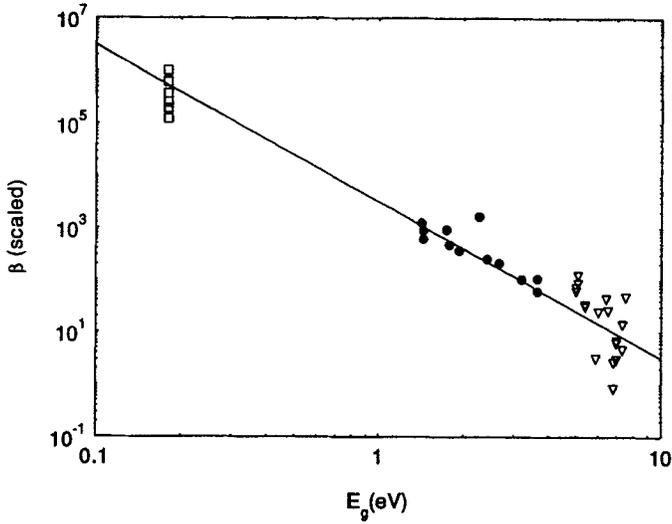
FIG. 6. Log-log plot of scaled  $\beta^*$  as a function of  $E_g$ . The straight line is of Eq. (51) showing the  $E_g^{-3}$  dependence. Adapted from Van Stryland *et al.* (1988).
