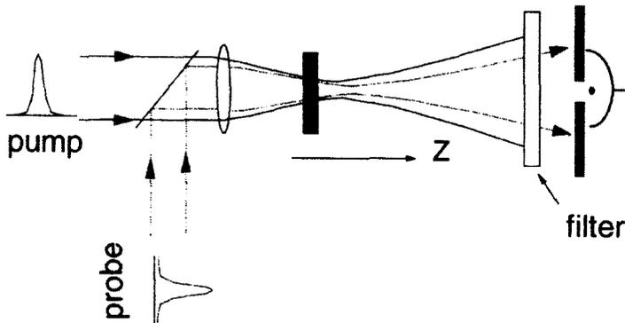
FIG. 21. Optical geometry for a two-color Z-scan. The filter blocks the pump beam. Adapted from Sheik-Bahae *et al.* (1992).
