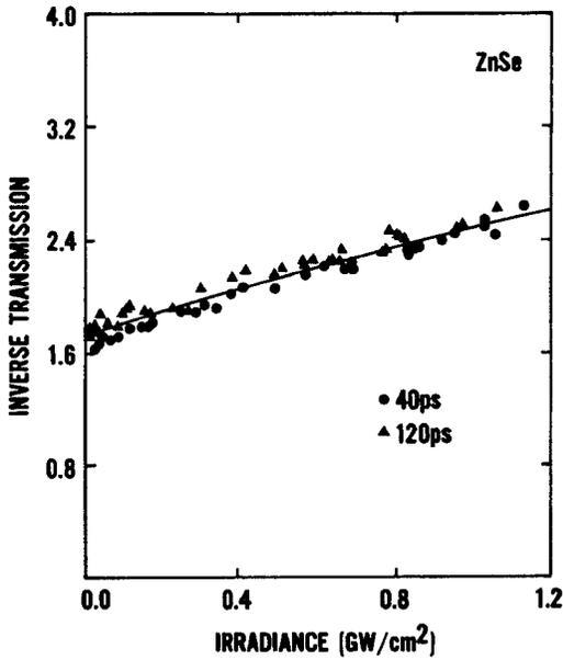
FIG. 14. Inverse transmittance as a function of irradiance of 532-nm picosecond pulses in ZnSe for two different pulse widths. Figure from Van Stryland *et al.* (1985a).
