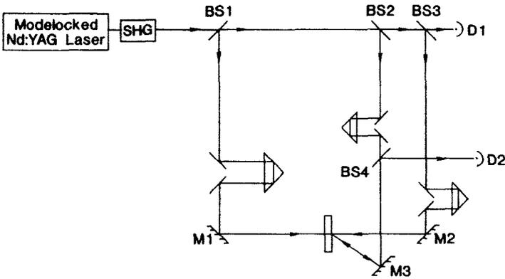
FIG. 16. DFWM geometry to allow temporal dynamics measurements. Detector  $D_2$  monitors the conjugate beam energy. Figure from Canto-Said *et al.* (1991).
