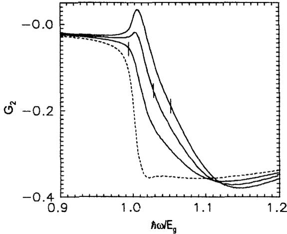
FIG. 11. Calculated dispersion function  $G_2$  for various injected current density levels. The dashed line is for passive material. The transparency point of each curve is marked with a vertical bar. Figure from Sheik-Bahae and Van Stryland (1994).
