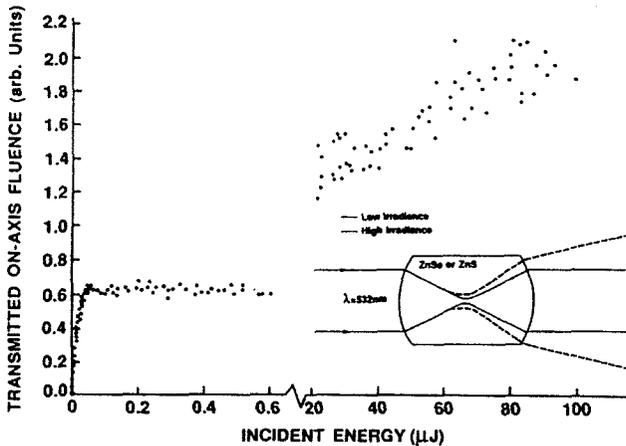
FIG. 25. Optical limiting data for the monolithic ZnSe lens ( $\sim 3$  cm long) shown in the inset for picosecond, 532-nm pulses as a function of the input energy as measured through an aperture approximately 2.5 m after the sample. Adapted from Van Stryland *et al.* (1988).
