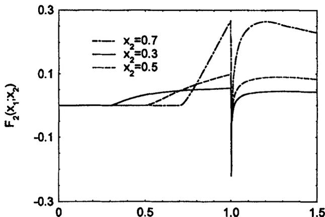
FIG. 4. The nonlinear absorption spectral function  $F_2$  showing the change of absorption at  $\omega_1$  due to three different photon energies  $\omega_2$ .
