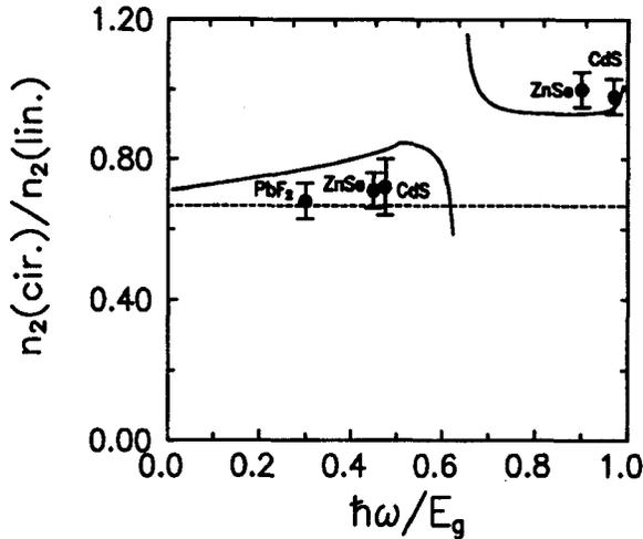
FIG. 10. The dispersion of the polarization dichroism of  $n_2$  measured using Z-scan. The solid line is from the three-band theory, and the dashed line represents the two-band model. The divergence near  $\hbar\omega/E \cong 0.65$  corresponds to the zero crossing of  $n_2$  (linear polarization) at that wavelength. Figure from Sheik-Bahae *et al.* (1991).
