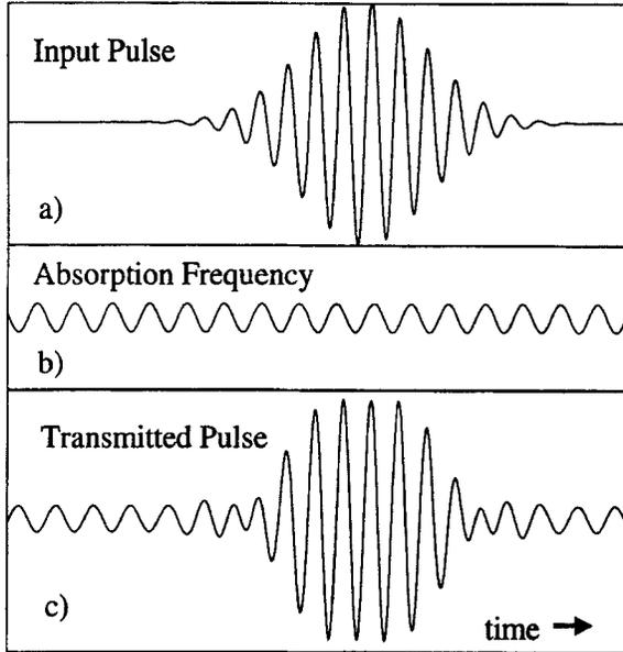
FIG. 1. Pictorial representation of the need for a relation between index and loss: (a) input pulse electric field in time; (b) absorption component in time. (c) (a) - (b). After Toll (1956).
