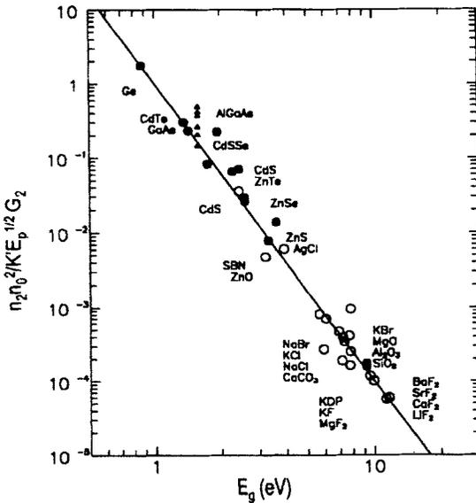
FIG. 9. Log-log plot of scaled  $n_2^2$  as a function of  $E_g$  showing the  $E_g^{-4}$  dependence (straight line). The AlGaAs data are taken from LaGasse *et al.* (1990), and much of the large-band-gap data are from Adair *et al.* (1989). Adapted from Sheik-Bahae *et al.* (1991).
