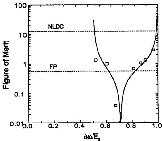
FIG. 24. Ratio of  $n_2/k\beta$  (switching parameter or figure of merit) as a function of  $\hbar\omega/E_g$ . The solid line is predicted from the two-parabolic-band model. NLDC stands for nonlinear directional coupler, and FP stands for Fabry-Perot etalon. Figure from Sheik-Bahae *et al.* (1991).
