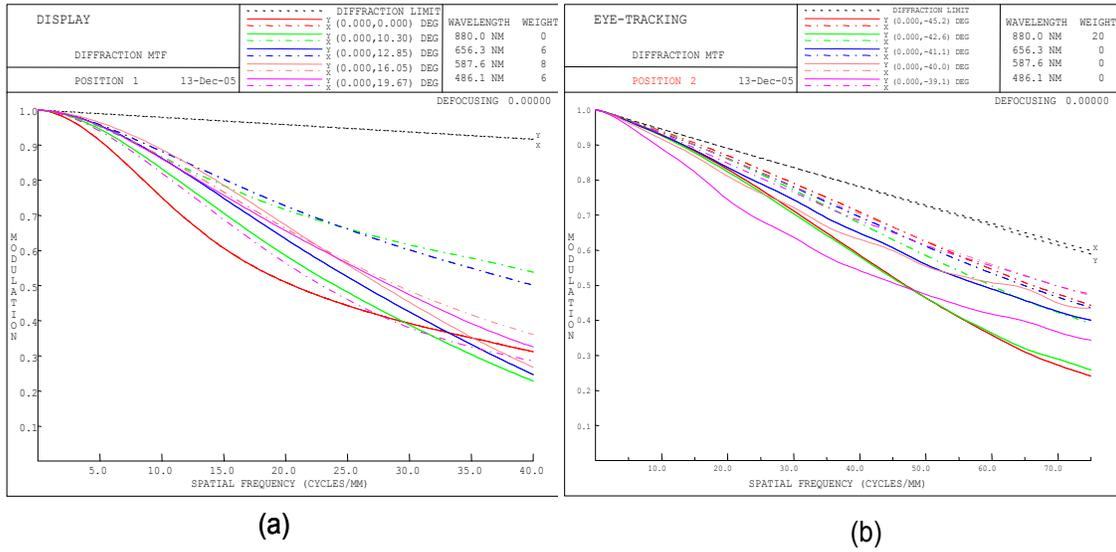
Figure 5: (a) MTF curve for the Display path (b) MTF curve for the Eye-Tracking path
