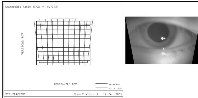
Figure 7: Distortion grid on the camera plane and trapezoidal distortion effect on eye image
