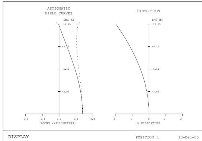
Figure 6: Field plots for the display path
