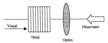
Fig. 1. Principle of multi-focus planes HMD.
