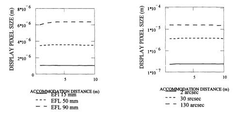
Fig. 6. Display resolution requirements: (a) Plot of the display resolution required as a function of the distance of accommodation L for three values of the focal length: 15 mm, 50 mm, and 90 mm. The stereoacuity threshold  $\eta$  is 30 arcsec in this computation. (b) Plot of the display resolution required as a function of the distance of accommodation L for three values of the stereo acuity threshold  $\eta$ : 2 arcsec, 30 arcsec and 130 arcsec; In this case the focal length is set to 50 mm.
