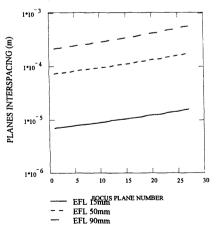
Fig. 4. Planes' interspacing as a function of the focus plane number for three different values of the focal length.
