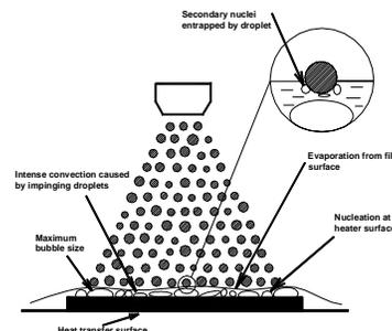
Figure 2. Spray Cooling Heat Transfer Mechanisms
