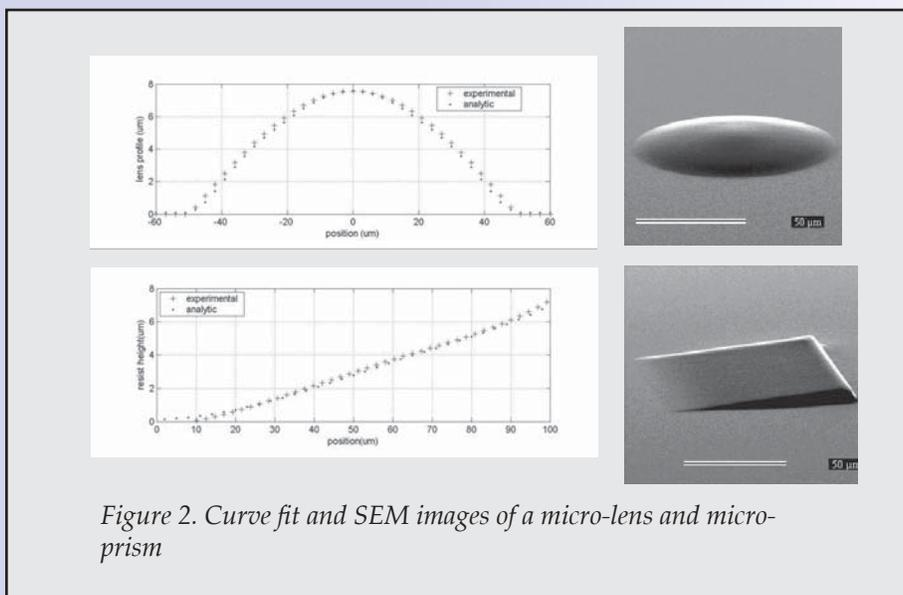
Figure 2. Curve fit and SEM images of a micro-lens and micro-prism
