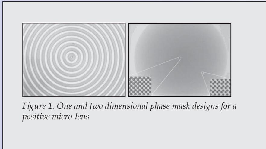
Figure 1. One and two dimensional phase mask designs for a positive micro-lens
