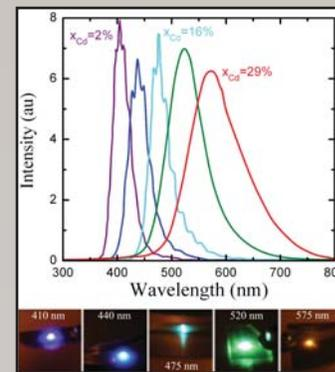
Figure 2: CL data and corresponding optical images from various  $\text{Cd}_x\text{Zn}_{1-x}\text{O}$  epilayers.
