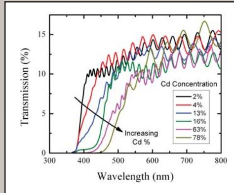
Figure 1: Shift in band edge as a function of Cd concentration.
