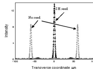
Fig. 3. CW simulations of control of multiple soliton generation by a small SH seeding beam. Nonlinear parameter corresponds to KNbO<sub>3</sub>
