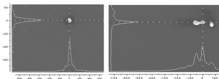
Fig. 1. Experimental results for normal incidence along the "b"-axis at 983.5 nm with the FW polarized along the "a" crystal axis and the SH along the "c" axis of a KNbO<sub>3</sub> crystal.
