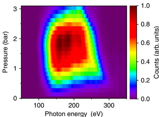
**Fig. 2** Pressure-dependent soft X-ray yield. Soft X-ray continua generated by polarization gating as a function of pressure in the neon gas cell. The spectra were recorded by an electron TOF spectrometer and corrected for the photoionization potential (21.6 eV) and absorption cross section of the neon detection gas. Photons with energy <100 eV were filtered out using a 100 nm tin filter
