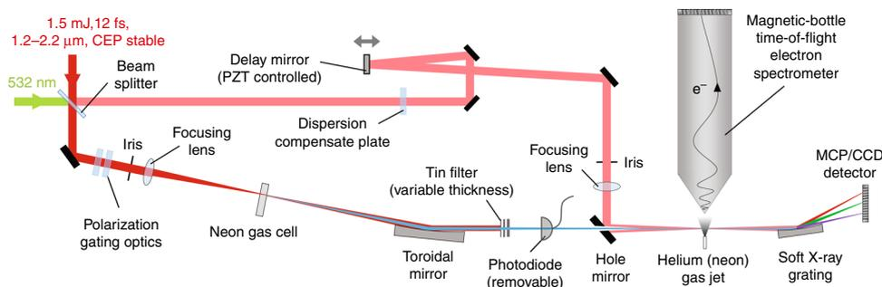
**Fig. 1** Experimental set-up. Schematic illustration for isolated attosecond X-ray pulse generation and characterization. CCD charge-coupled device; MCP microchannel plate, PZT piezo-electric transducer
