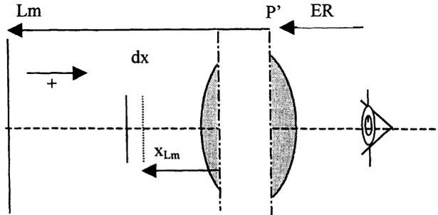
Fig. 2. Basic layout of the imaging optics in a head-mounted display.
