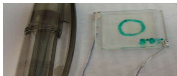
Figure 6 An 8 μm thick polymer dispersed liquid crystal in a twisted cell (T-PDLC) sample next to a pen as a size reference.
