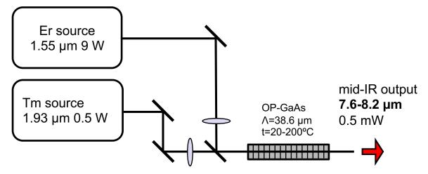
Near-IR power: 9 W + 0.5 W Mid-IR power: 0.5 mW Conversion efficiency: ~ 10<sup>-4</sup> W<sup>-1</sup>
