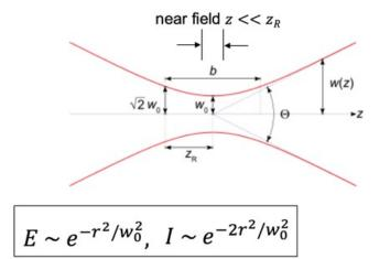
The DFG beam at  $\omega_1$  has the beamsize  $w_0/\sqrt{2}$
