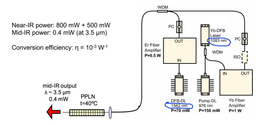
Experimental setup for the 3.5-µm DFG source based on mixing the amplified outputs of two DFB lasers in PPLN. DL, diode laser; ISO, optical isolator; PC, polarization controller; WDM, wavelength division multiplexer.
