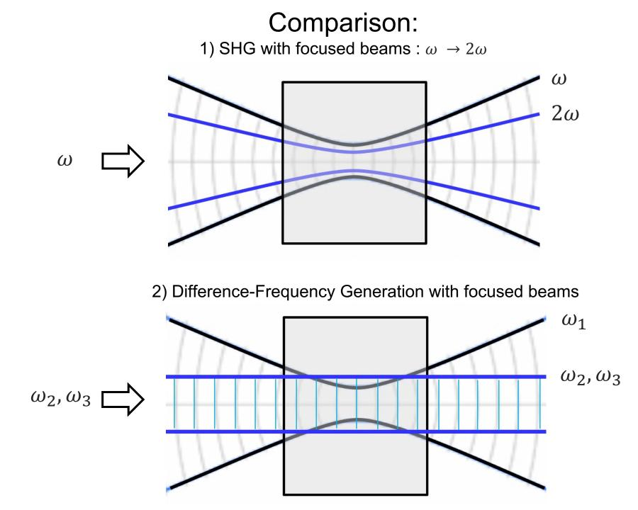
The Gaussian fundamental beam (solid line) and its 2-nd harmonic (dashed line) propagate in a similar way (and have the same Rayleigh length  $z_R$ ). The radii of curvature coincide since
