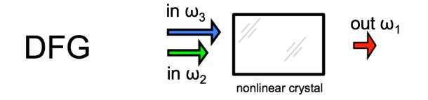
Assume that the  $\omega_3$  wave and  $\omega_2$  wave are strong waves and are undepleted by the nonlinear interaction, so that we can treat  $A_3$  and  $A_2$  fields as being essentially constant.
