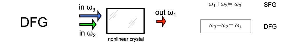
$\omega_3$ ,  $\omega_2$ , and  $\omega_1$  are the so-called pump, signal and idler waves by definition  $\omega_3 > \omega_2 > \omega_1$
