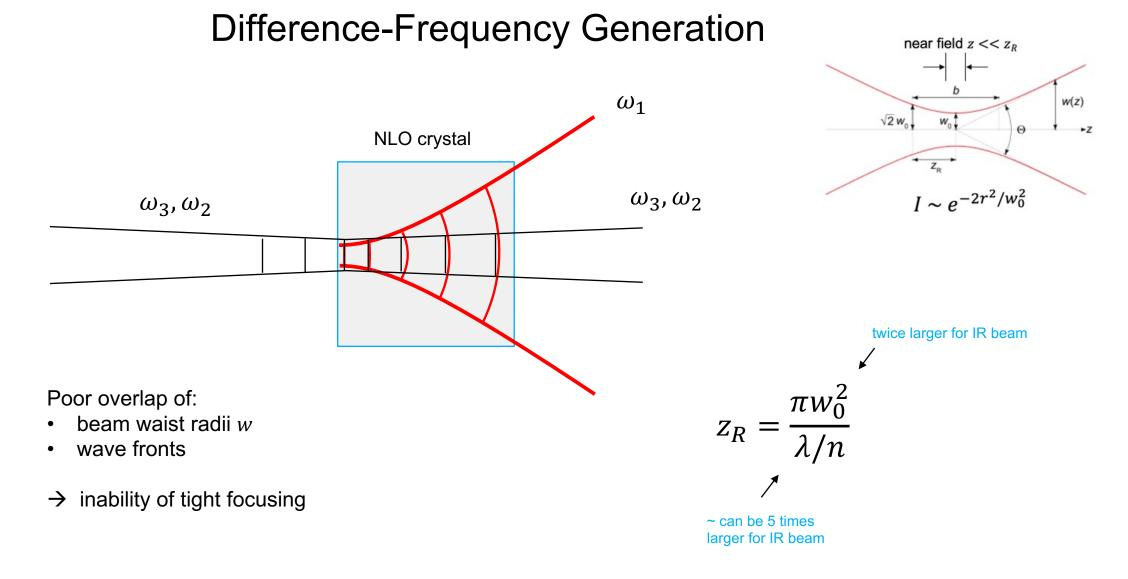
Because of the poor overlap, one can not focus the pump tightly – need to have the pump beams to be such that for the genearted IR beam ( $\omega_1$ ):  $z_R$  > crystal length.
