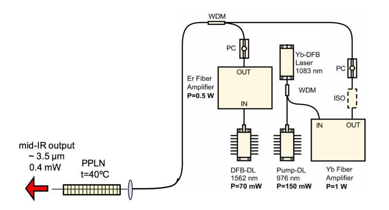
Experimental setup for the 3.5-µm DFG source based on mixing the amplified outputs of two DFB lasers in PPLN. DL, diode laser; ISO, optical isolator; PC, polarization controller; WDM, wavelength division multiplexer.
